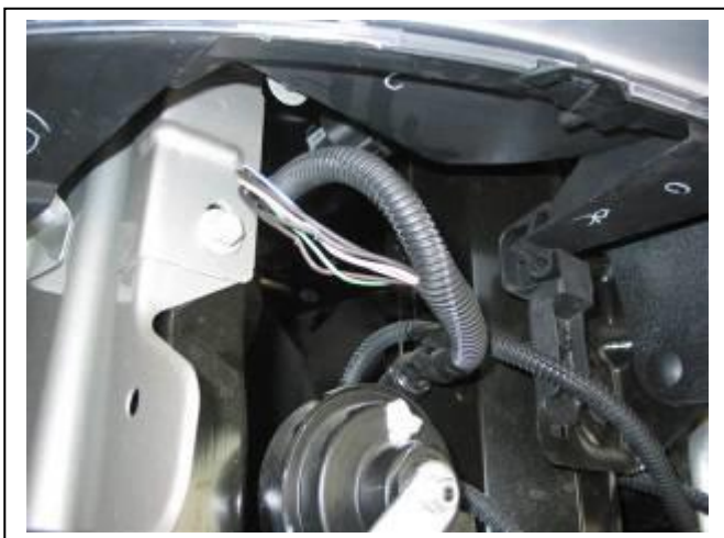
Figure 7: Wiring harness under driver's headlamp
