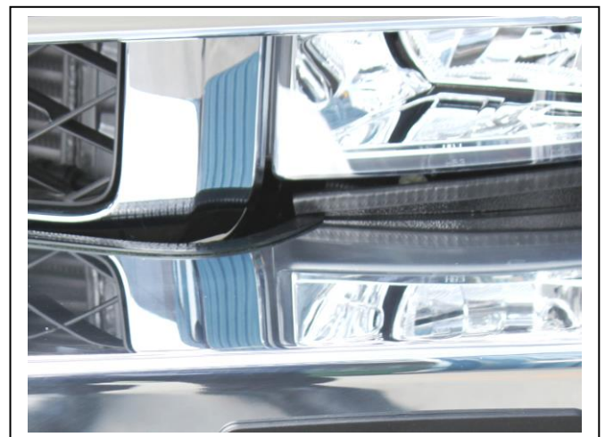
Figure 8: Point on bumper alloy infill meets 6mm clip lock trim.
