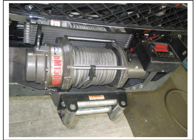
Figure 4: Placement of winch in mount
