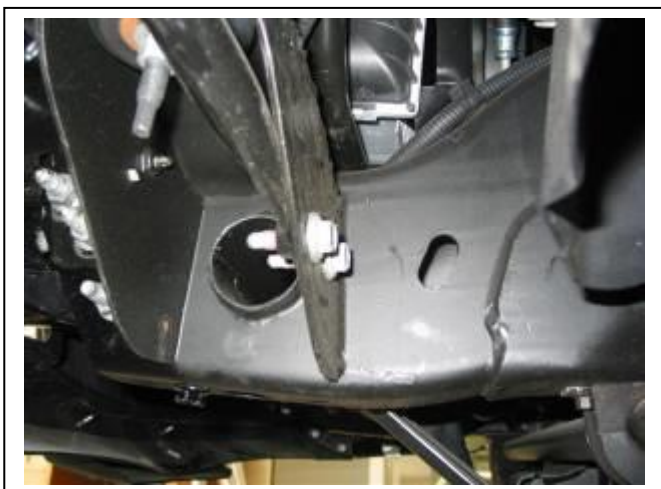
Figure 1: Stay mount to chassis, two 15mm bolts
