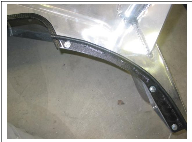
Figure 9: 6mm clip lock trim protrudes past alloy infill and is locked down when bolts are tightened.
